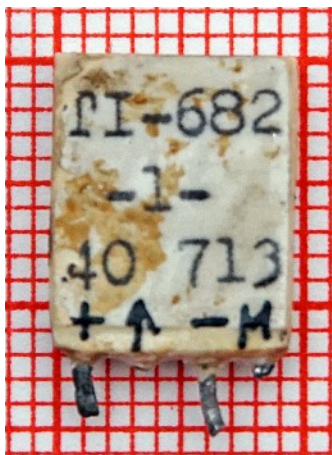
TI-682 subminiature bug. Shown enlarged in a 1mm grid.
