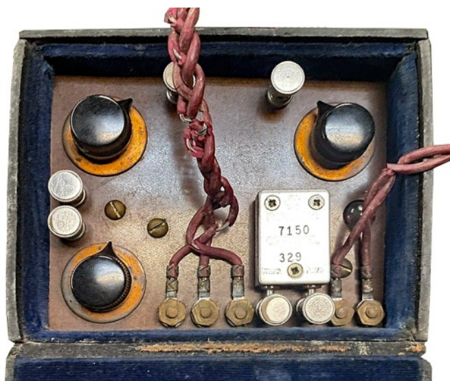
Transmitter top view showing controls and connections.
