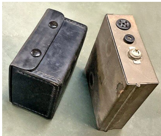
Transmitter and battery box ready for transport.
