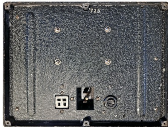
Bottom view of Supply Unit Vibratory No. 14 showing 4-pt output socket, 6V input and fuse holder.
