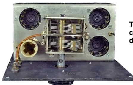
Top view of E 75 chassis with valves detached.
