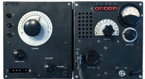
The S 85/14 was in combination with its companion receiver E 75 (left), known as SE 85/14.
