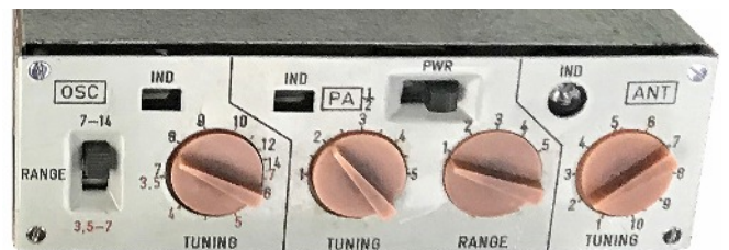
Front panel view of the S-50B transmitter unit.
