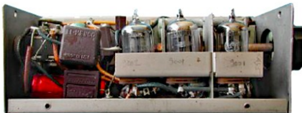
Left and right hand side views of Mk.18 showing receiver section with three miniature type valves (photograph above) and transmitter (photograph below). Note the 4mm socket in the left hand corner of the bottom picture for connecting the aerial.
