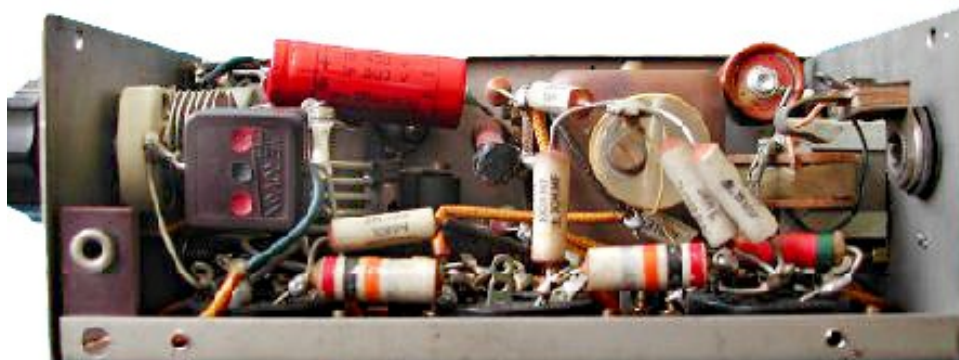
Left and right hand side views of Mk.18 showing receiver section with three miniature type valves (photograph above) and transmitter (photograph below). Note the 4mm socket in the left hand corner of the bottom picture for connecting the aerial.
