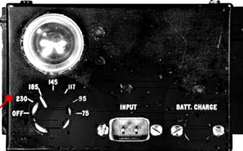
**The 12V accumulator of a RS-13 station was charged by a separate AC powered charger unit.**
