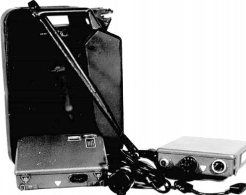
**The 'Jerrycan' agents set was an AC mains powered version using an AC mains power unit in place of a battery box.**
