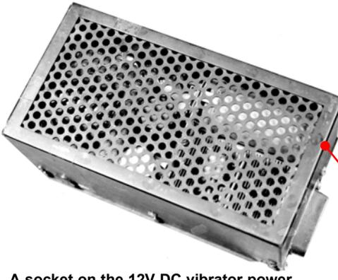
**A socket on the 12V DC vibrator power unit above slid into contacts at the left hand side of the RS-13 transmitter.**
