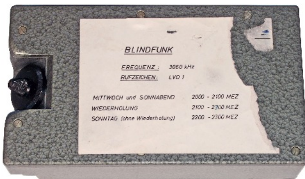
Bottom view of an Uhu receiver showing tuning control knob. Note the glued time scale and frequency of a 'blind transmission' number station operating on 3060kHz.
