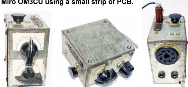
Detail view of OK1AU agents transmitter replica built-in Morse key, ingeniously constructed by Miro OM3CU using a small strip of PCB.
