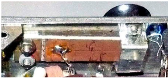
Detail view of OK1AU agents transmitter replica built-in Morse key, ingeniously constructed by Miro OM3CU using a small strip of PCB.
