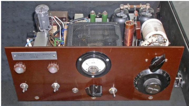
Front panel view of the Burza replica (above). Similar to the destroyed 1944 original, it was built on a wooden baseboard with a Pertinax front panel, using as much as possible period components. The maker of the Burza replica was Zygmunt Seliga, SP5AYY, who also took the photographs.
