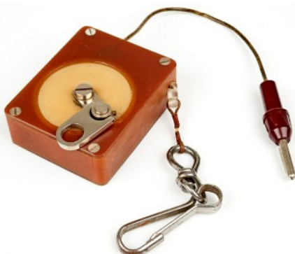
Neon mains voltage tester (right) and reel antenna (left) were issued with the Sirius station and packed in the accessories case. Both units were probably inspired by similar devices which were standard issue with most of the post-war British agents sets.
