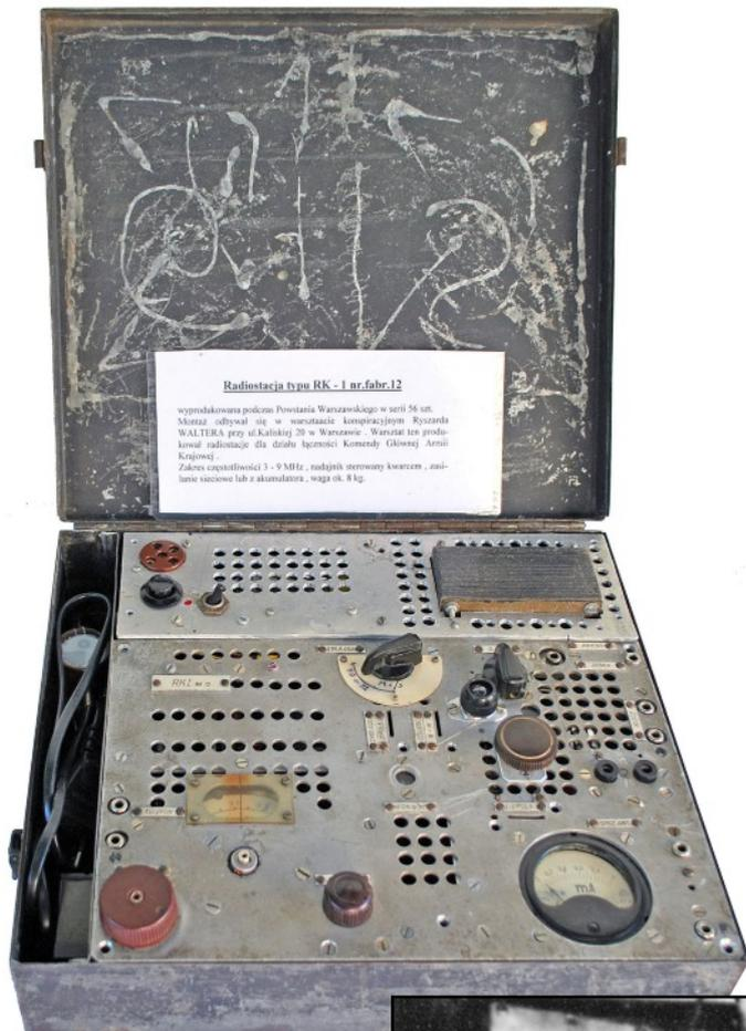
The RK 1 on the photo above was a partial rebuild using an original metal box and almost bare donor set, fortunately still with most of the engraved inscription plates. The AC mains power supply unit at the top was a reconstruction. The meter in the right hand bottom was not original, replacing an original rather large Aerial Coupling knob.
