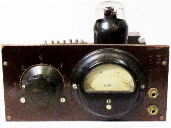
Miro Hornik, OM3CU, originally built a NK-1 transmitter replica on a baseboard with Paxolin front panel incorporating a meter (above and top right). He was later informed that an AvoMinor I multimeter was issued to the wireless operator and accordingly changed his replica as pictured on page 1.
