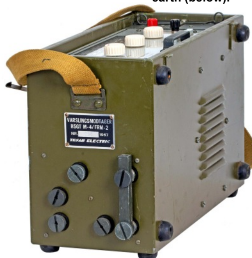
Left hand side view with connections to aerial and earth (below).
