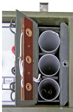
Right hand view of front panel with battery compartment opened (left).
