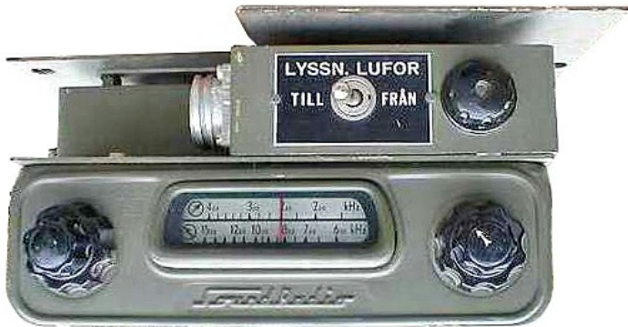
Front panel view of MT 920 E fitted on a different frame with on/off switch and fuse placed on top of the receiver (Above). This was a variation for installation in combat vehicles.
