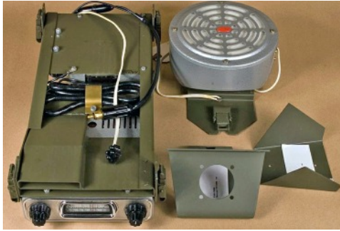
Standard frame for Mt 920 with separate loudspeaker and aerial brackets (Above and right).
