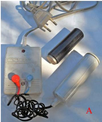
In winter time, under extreme low temperatures, the battery pack fitted in the charger case and worn on the body, was connected to sockets at the side of the radio (below).
