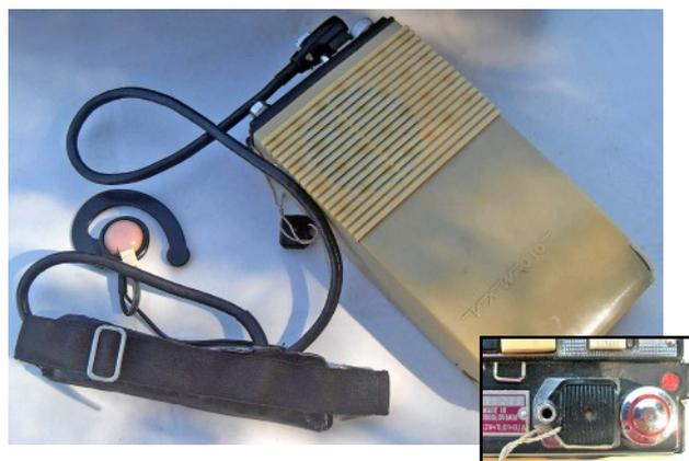
VXW 010 with throat microphone and earphone. When not in use it required a dummy plug with shorting pins (Inset).
