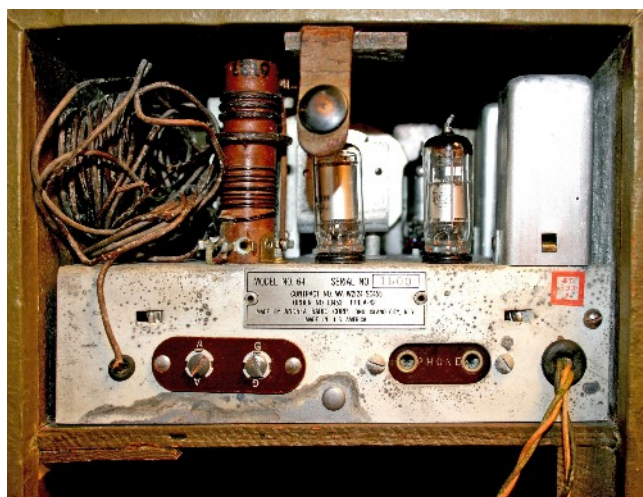
Detail view of the receiver chassis with coiled-up aerial wire (left).
