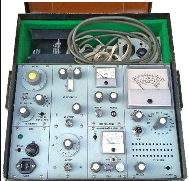
For regular maintenance and repairs of the VXW 100 (and many other VHF FM radios) a test set Tesla PSK 92 was used.
