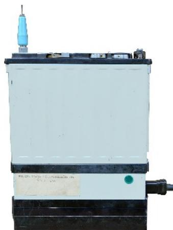
**VYN 005 battery charger and rechargeable battery fitted at the bottom of a VXW 100 (left).**
