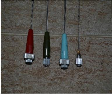
For each frequency band was a set of three aerials (long, short and a short wire aerial). These were distinguished by a coloured coded base. From left to right: 34, 45, 80 and 160MHz.
