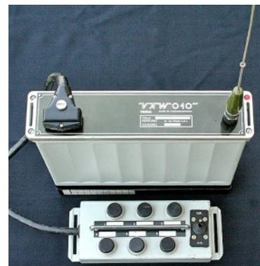
A spin-off from the VXW 100 was the VAW 010, a transmitter only, used for remote control of industrial and agricultural applications (above).
