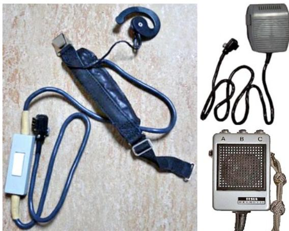
For (inconspicuous) hands free operation of the radio a throat microphone/ptt button and a short wire aerial could be used (left). QN 618 05 was the VXW 100 standard microphone (top right); the PX 25 microphone was primarily issued with the PR 11 (bottom right).
