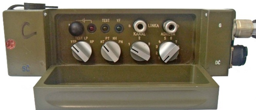
Seismic Sensor unit (SČ)
