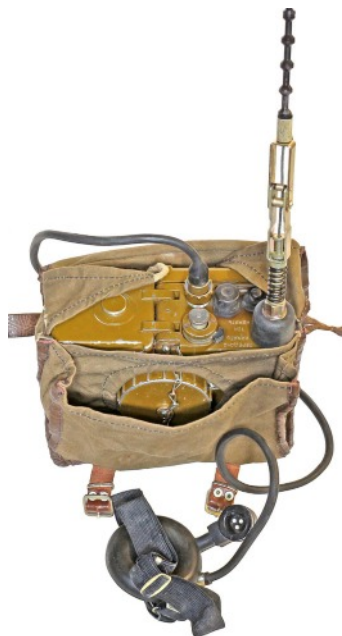
Russian R-352 special forces VHF FM radio used for activating and exploding the BON.
