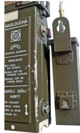
KD-1/SB connected via a multi-core cable to the handset socket of a standard RF-10. It was suspended at the side of the set (right). The KD1/SB transmitter was actually a tone code generator for detonating the charge. The firing was initiated by rotating the switch on the top of the transmitter to the 'Detonate' position. One of the three designated channels must be set on the RF-10 to match the specific receiver(s) of the SBON kit. In a kit were 4 receivers.
