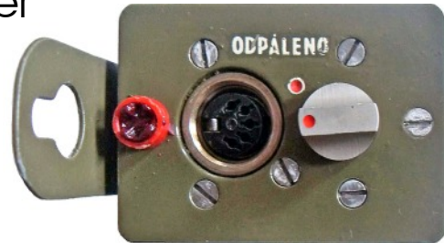
Top view of KD-1/SB with detonate switch and socket to connect a RF-10.
