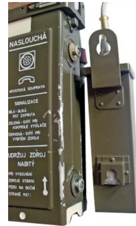
Top view of KD-1/SB with detonate switch and socket to connect a RF-10.
