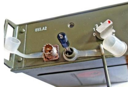
Detail view of aerial socket and time fuse pin. Pulling out the pin activated the booby trap and the time lock of the radio (if both were activated). When these modes were active and the receiver unlocked, a mercury tilt switch was activated. An explosion occurred when the device was tampered with.
