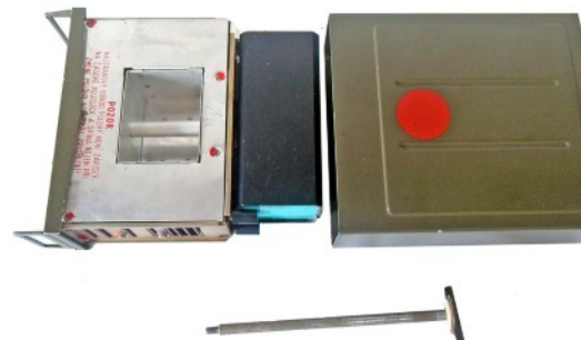
Top view of opened PR-1/SB showing the actual receiver (without explosive charge), rechargeable battery, cover and back cover screw.
