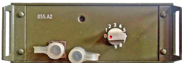
Front panel view of PR-1/SB receiver showing code switch, (covered) aerial socket and time fuse pin.
