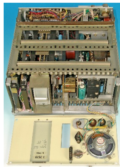
32620 with top and side covers removed showing the internal construction.
