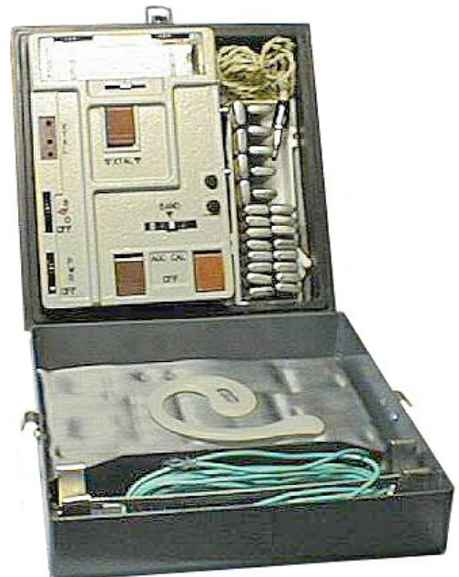
Seja with crystal box and accessories in container. It may be speculated that an associated transmitter was stowed in the empty space in the lower part of the container
