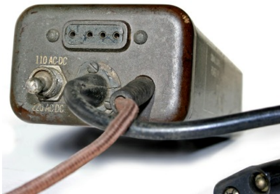
Top view of the RBZ Power Pack showing the mains voltage switch, socket for connecting the RBZ, headphones cable/plug and mains cord.
