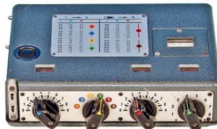
The West German FS-7 transmitter was part of the SP-15 station which was comprised of a FS-7, FE-10 receiver, AC mains power unit, DC power pack and RT-3 high speed Morse keyer (See Chapter 56).
