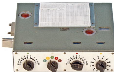
The SE 25, also known as 'Elbe' was an East German agents transmitter. It was used in combination with a NE 25 AC mains power unit or a 12V DC transverter, and a high speed Morse Keyer 'Geber E' (See Chapter 60).
