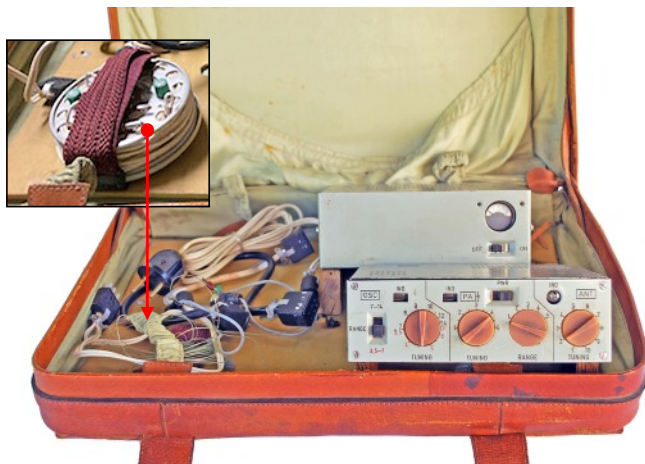
General view of the S-50B Polish suitcase with the transmitter and AC mains power supply unit in position. Missing in this photo is the synthesiser and an unknown type of high speed Morse keyer.
