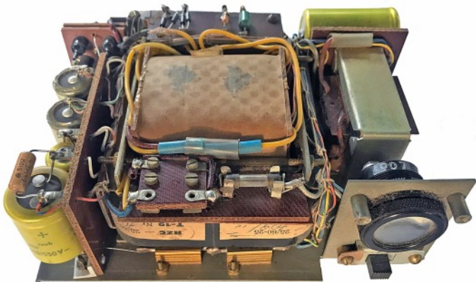
Front panel view of AC mains power unit with its cover detached showing meter and on/off switch.
