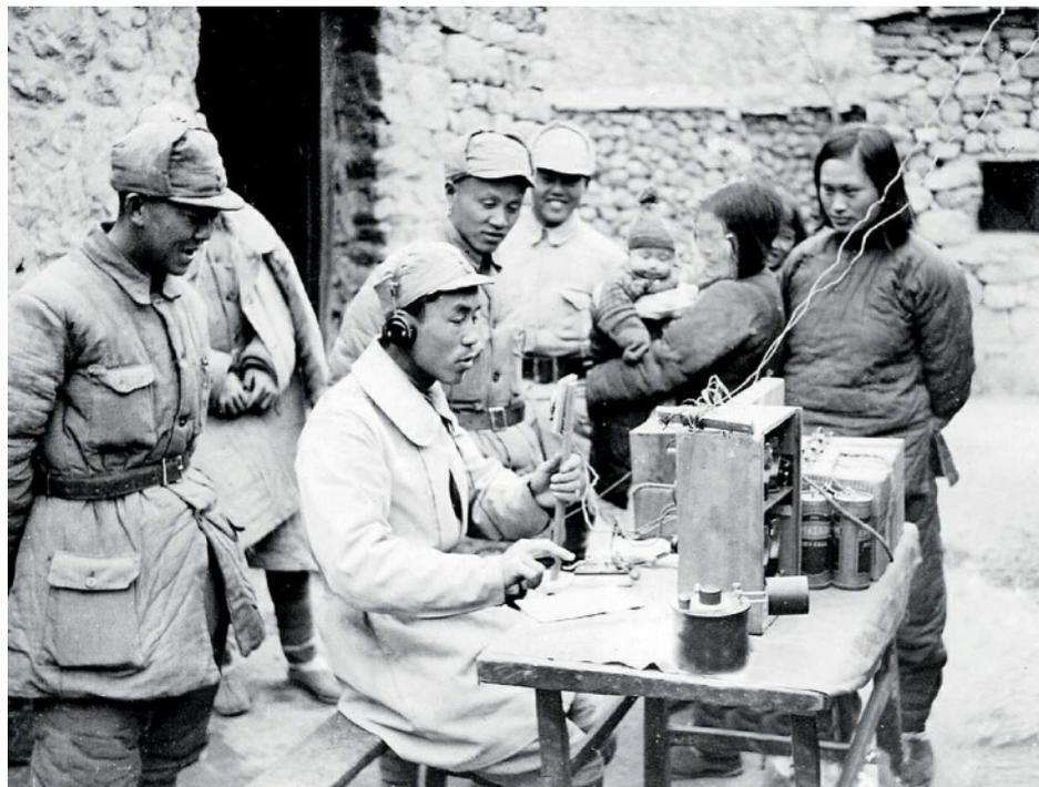
This photograph shows Michael's wife Hsiao Li looking on intently as an operator reads a message and sends it via the key. It also shows how the transmitter and receiver units were mounted one above the other in a protective wooden frame suitable for transport in a back pack. Two rather untidy wires diverge up, presumably to a dipole antenna. Their first child is peaceful in the arms of a nurse. Michael Lindsay will have taken the picture.
