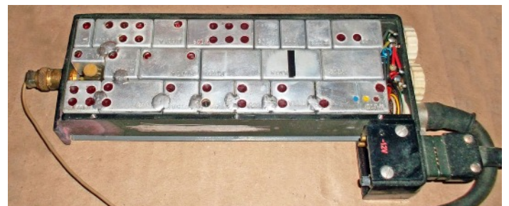
Internal view of a Hvězda 5a showing the modules embodying all the electrical circuits, held in an aluminium frame.
