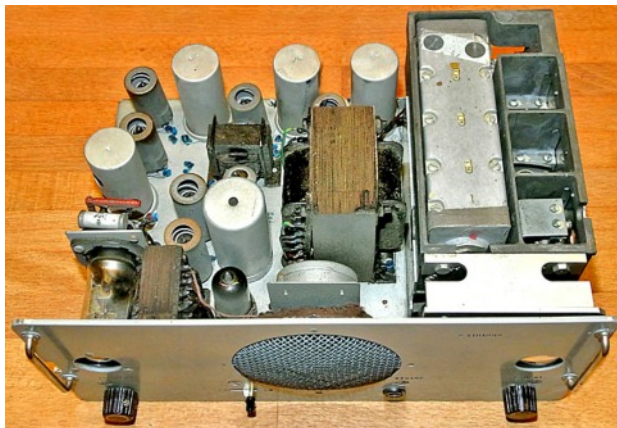
Top view of Vltava chassis showing the Fug 17 front end unit (right) and IF strip (rear and left).
