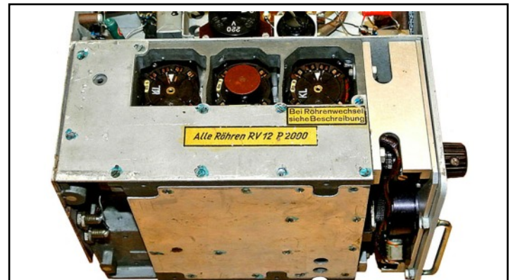
The RF front end of Vltava was originally part of a Luftwaffe FuG 17. This unit was also used in the Ukw.E.d1 (part of Wehrmacht Fu7 vehicle set for communication with aircraft), and Kriegsmarine Lo10uk39, the latter with a slightly different frequency coverage.
