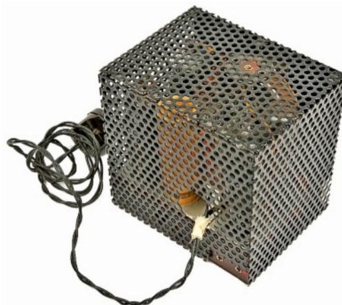
**Rear view of the MA 444 Svenskesuperen. Note the headphones sockets at the bottom right. The aerial was connected to a socket at the top.**
