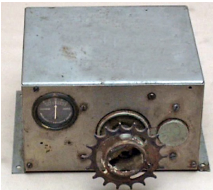
The Mk.VII hand generator pictured here was modified by a Norwegian Milorg group to be operated by a bicycle.
