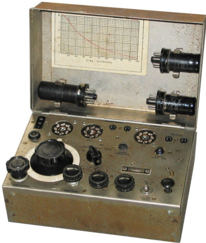
Mk.VII 'Paraset' with valves fitted in clips in the lid.
