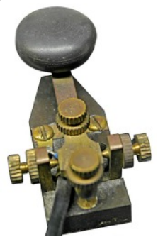
Miniature Morse key issued with the KT-023 transmitter.
