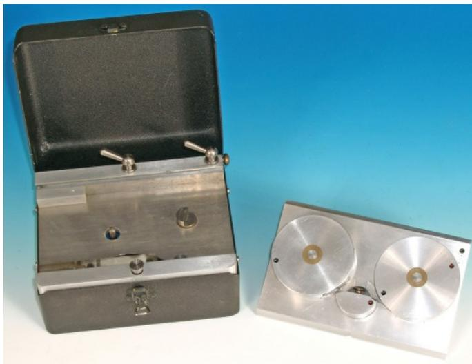
French high speed keyer in transport case (left) with metal tape spools and top deck detached. (right).
