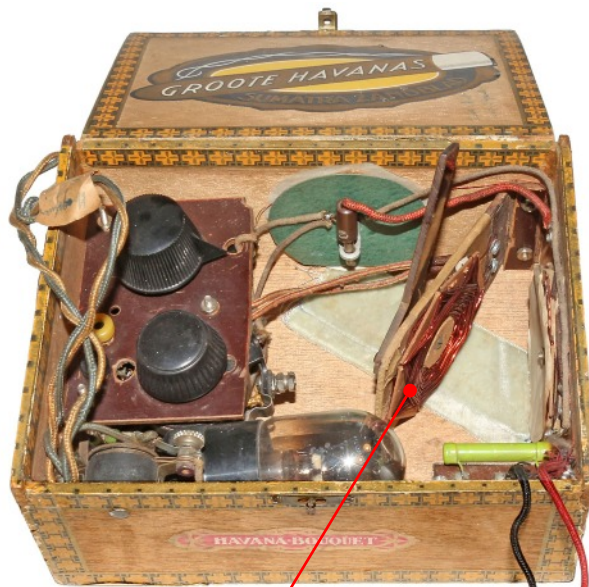
Midget receiver #7A with loosely coupled tickler coil.
