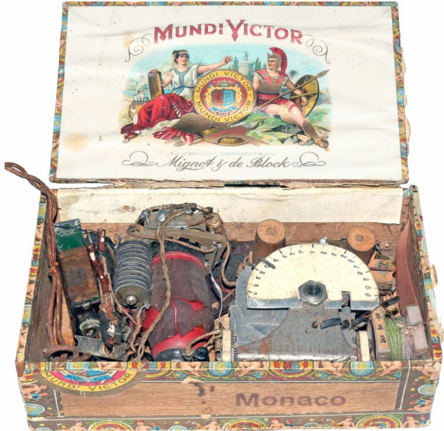
Midget receiver #7B built into a Mignot & de Block 'Monaco' cigar box.
