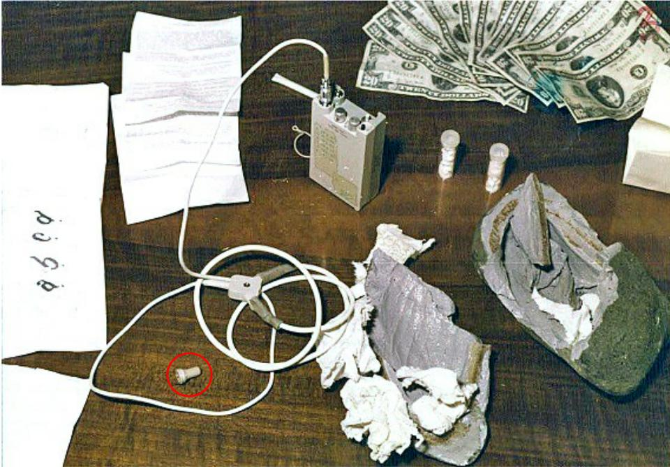
Close-up photograph of an SRR-100 receiver (as pictured in large format on the previous page) taken from a captured USA agent by the KGB. Note the Phonak hearing aid type earpiece and two small plastic containers with spare mercury cells.
