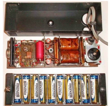
Top view of Dunaj B receiver with cover removed. The down converter was located under the screened compartment on top right of the main chassis.
