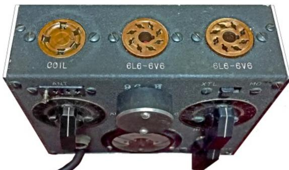
Top view of CMS-T showing valves and coil sockets.
