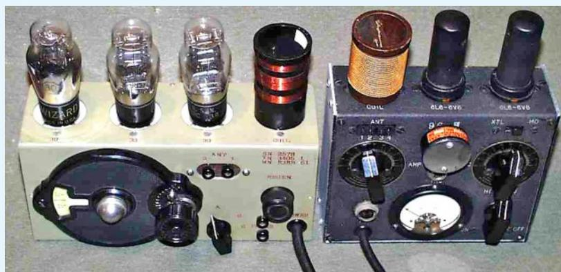
The unknown 3 valve receiver compared to a CMS-T transmitter.
