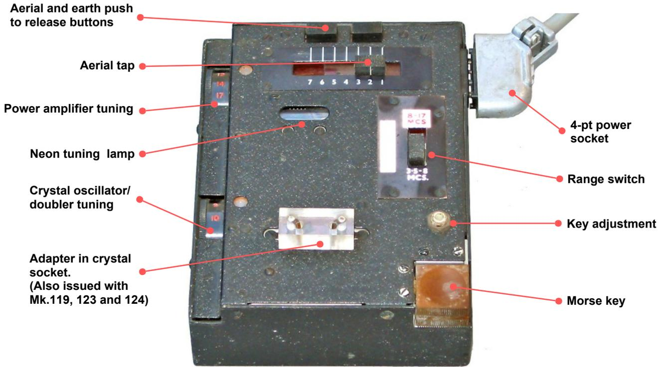
Function of controls Mk.217 transmitter unit.
