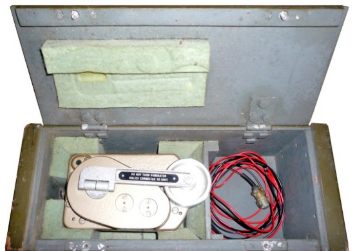
Top view of the opened transport case with Mk.819 generator and cable in position. It may be speculated whether a carpenters clamp and a base plate had been stowed in the nearly empty compartment at the right.
