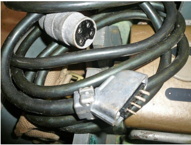
Cable connecting the Mk.818A (round socket) to a Mk.217 transmitter. (4-pt rectangular plug)
