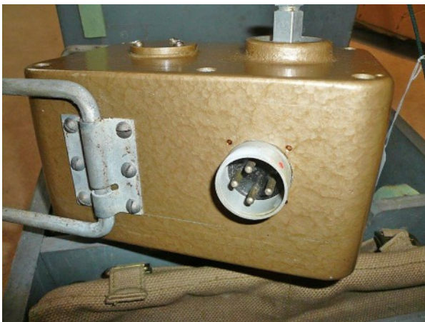
Side view of generator showing the round 4-pt plug
