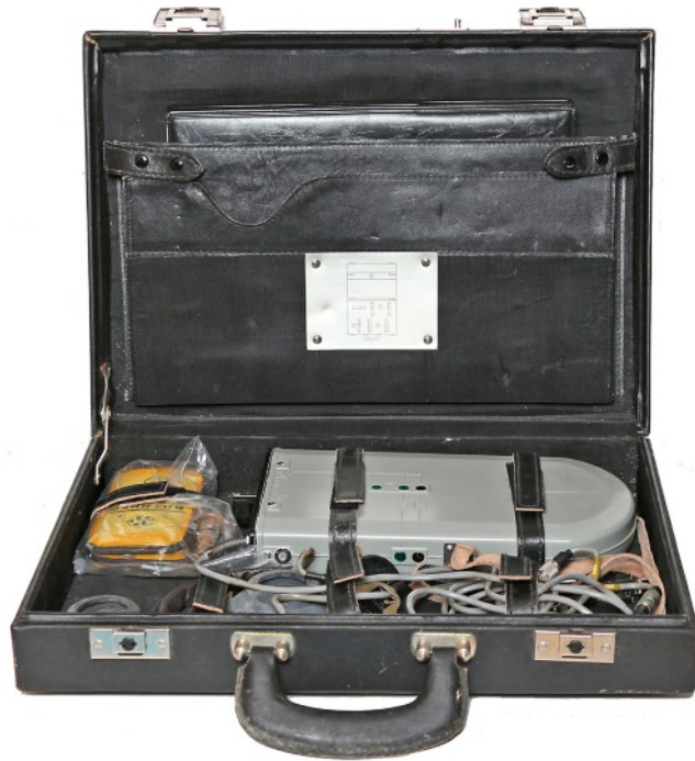
Internal view of attache case showing arrangement of MRK-1 and accessories.
