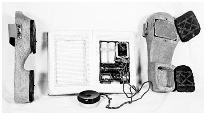
**General view of the book radio with associated clogs. The circuit was a single valve detector with reaction (cathode trapped type reaction -ECO type). A miniature bell transformer provided the filament supply. High tension voltage was obtained directly from the 110 volt mains supply through a VR92 miniature diode rectifier. Voltages could fluctuate anywhere between 70 and 130 volts. The single earphone was always kept apart from the receiver hidden in a hollowed clog.**
