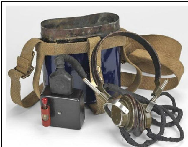
Detail view of the crystal receiver hidden in a modified pattern 37 water bottle.
