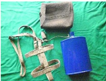
A crystal receiver constructed by N. Norris, a prisoner of war in Stalag III D near Berlin, was hidden in a pattern 37 water bottle. The bottle was modified and had a separate top section which could be filled with water. Along with the pouch nobody would suspect its authenticity. The first crystal detector unit was obtained from a French prisoner and a second from a German sentry in exchange for cigarettes. It had a coil tuner; a good aerial and earth were essential for reception.
