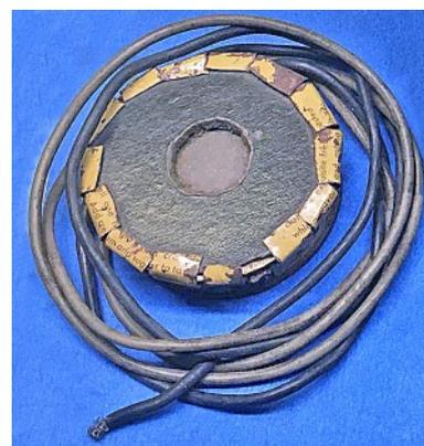
The earphone was made from an empty Nescafe tin, a piece of thin flattened tin as diaphragm, plus wire and a magnet from an electric razor.
