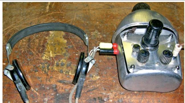
Another fine replica was constructed by Stefano Bianchini and Antonio of [www.usarmy1944.com](http://www.usarmy1944.com), based on the N6CC design and circuit. Vintage components were used throughout; the frequency range was changed to cover 6-18MHz
