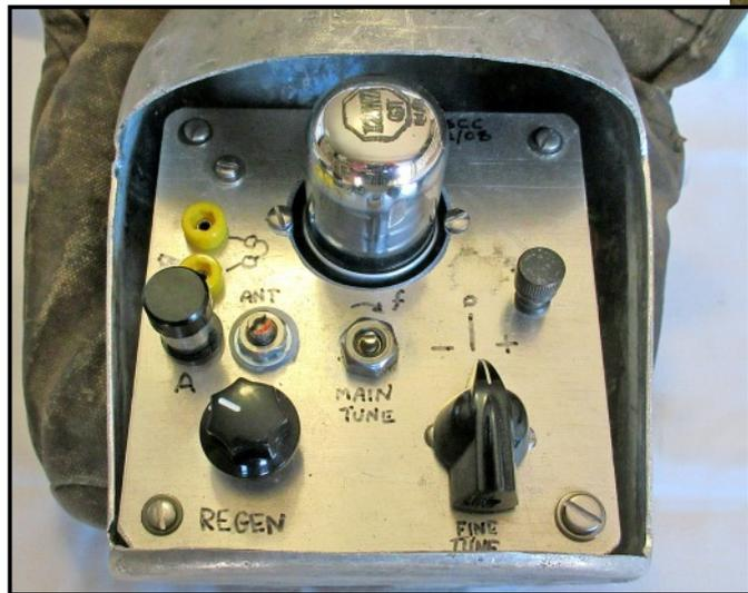
Close-up top view of Tim N6CC's replica of the PoW canteen radio (above).
