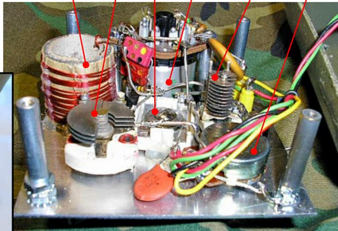
Bottom chassis view of N6CC's canteen radio. (above) For main tuning a mica compression trimmer (C1) was used, adjustable by a screwdriver. Fine tuning (C2) and aerial coupling (C3) was accomplished by two small variable condensers. The coil was wound on a piece of 1-inch bamboo.
