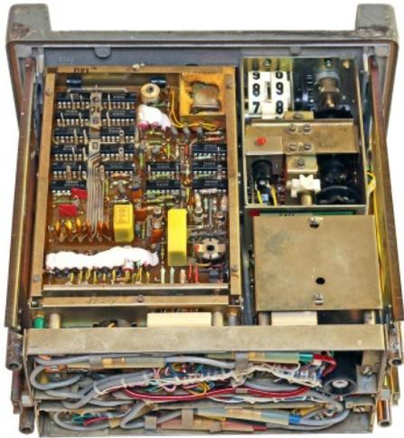
The UFT-435 was built extremely robust and rugged to withstand harsh field conditions. The operating temperature range of - 20°C to + 50°C and the degree of protection IP 54 (splash proof) secured the operability even in heavy rain and mud. The serviceability of the equipment was excellent. Individual modules could be folded out, allowing measurements directly on the circuit board.
