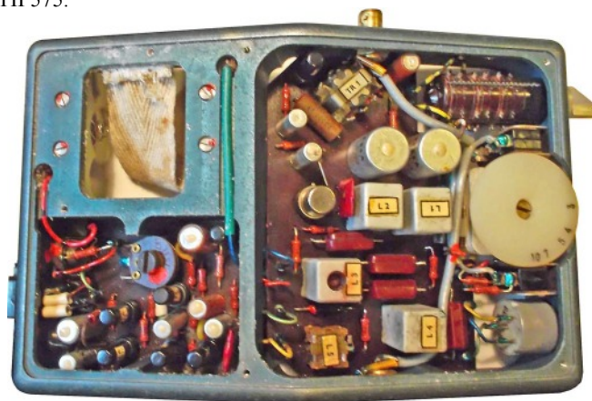
View of the Labe A receiver with top and bottom covers removed. The receiver was constructed in a die cast frame, using two printed circuit boards.
