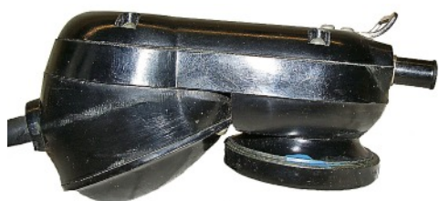
Peculiar shaped handset with PTT button on top. The B series had a different model handset. (See photo right)
