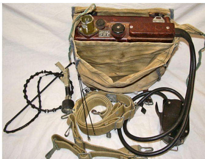
SHR-4P B Series which appeared to be similar to the O2R2 but with a different type of handset. Note the curled up Kulikov aerial
