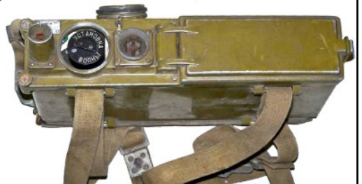
R-116 portable VHF AM transceiver, covert name 'Lily of the Valley'. Frequency coverage 48.65-51.30MHz in 10 channels with 294 kHz spacing. 60mW RF output. 1km range.
