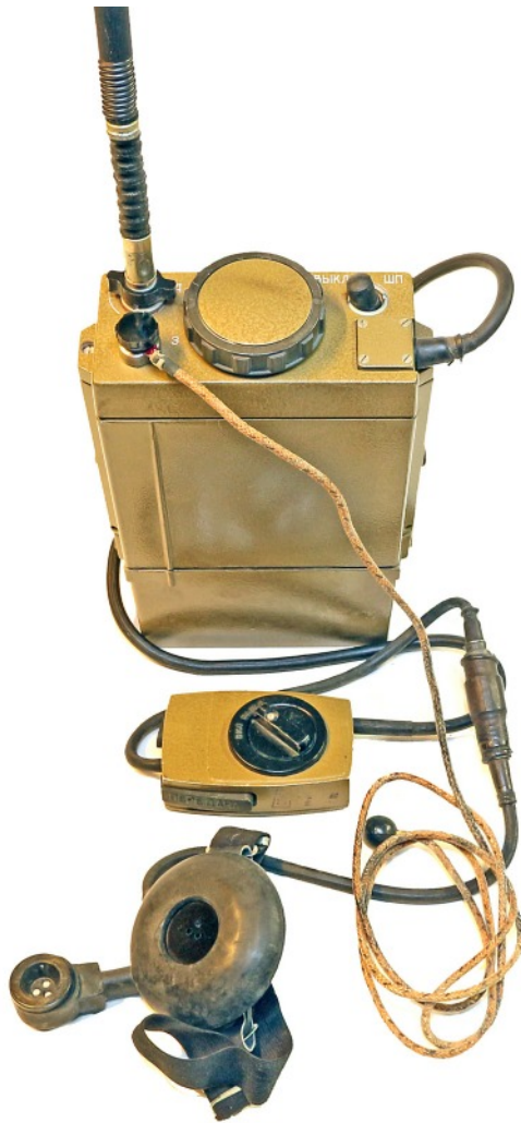
R-392 with Kulikov aerial, counterpoise wire, remote control unit and cheek microphone/headphone assembly.
