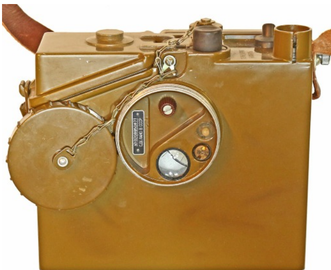
Side view of parent set, R-126, with opened protective cap. Note tuning control and frequency dial with a lens.
